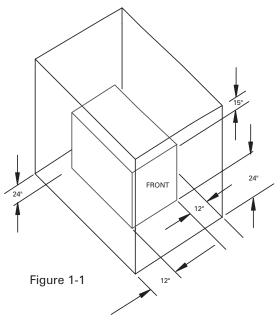
(NOTE: The Munchkin is rated at zero clearance to combustibles.)
